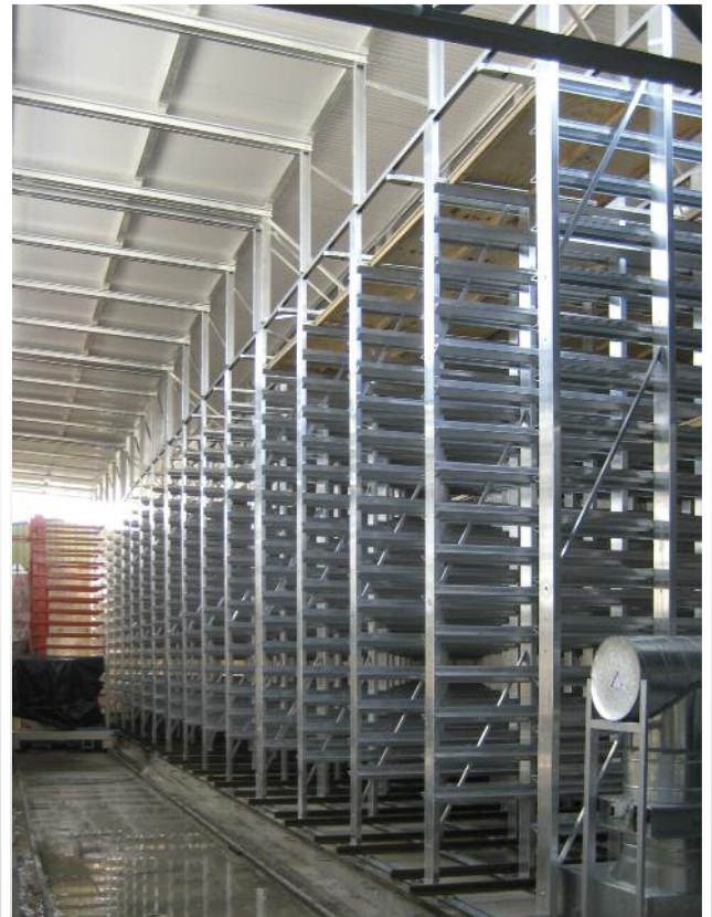
Secure storage and removal from storage by the finger car – the high lateral bead of the pallet support, with its continuous lateral guide, prevents collisions with the aluminium posts.
