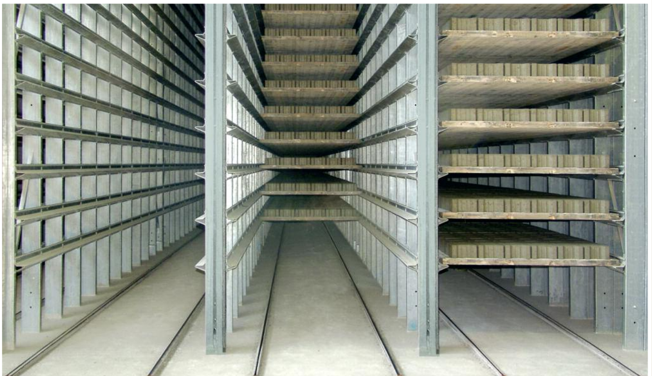
Curing chambers by HS Anlagentechnik are distinguished by their extremely high dimensional and fitting accuracies, parallelism and stability.
